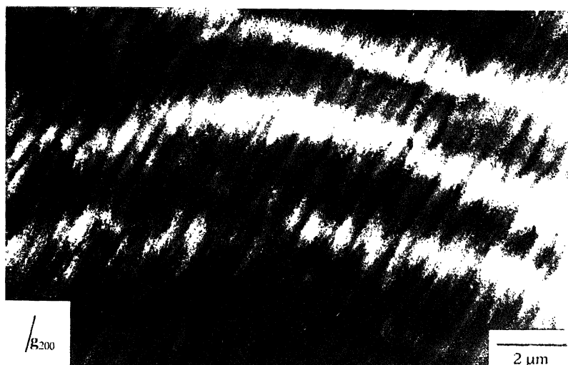
Figure 6. 200 dark field image of an InP– \text{In}_{0.53}\text{Ga}_{0.47}\text{As} –InP sample. Bright and dark bands represent changes in thickness of the \text{In}_{0.53}\text{Ga}_{0.47}\text{As} quantum well, which has an average thickness of 5 nm. (Courtesy of I. K. Jordan, unpublished work.)
