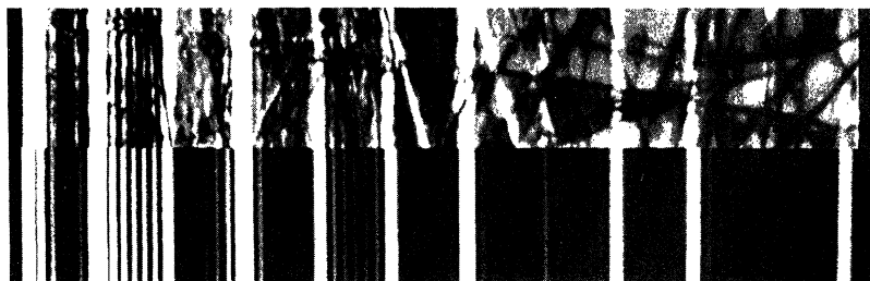
Figure 5. 200 dark field LACBED pattern from a 19.2 nm InP–11.1 nm \text{In}_{0.53}\text{Ga}_{0.47}\text{As} superlattice in the range 0.03 < s < 0.4 \text{ nm}^{-1} . Top, experimental; bottom, simulation; s increases left to right. (Courtesy of I. K. Jordan, unpublished work.)
